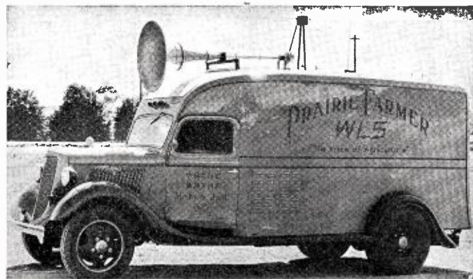
WLS MOBILE UNIT —This short-wave portable equipment, just completed by WLS, Chicago, consists of a 100 watt portable transmitter, a 30 watt mobile set and two pack transmitters, as well as public address system and field strength measuring equipment. Camera and sound recording apparatus are to be added. A roof hatch permits the announcer to stand upright in the truck, designed by Tom Rowe, chief engineer.
