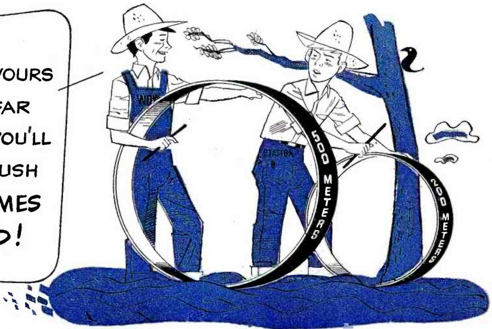
HERE'S the explanation: Natural and man-made obstacles impede the progress of radio waves. Long waves (low frequencies) are impeded much less than short waves (high frequencies) and hence go much farther with less power than shorter waves.
