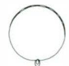
Figure 5B Properly Phased Tee Divider -10 kHz Pattern vs. Carrier Pattern r = .9995
