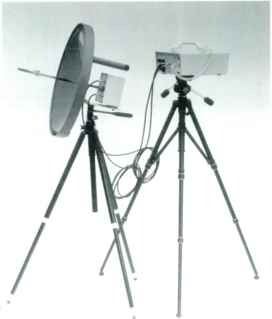
Portable simplex video/audio electronic news-gathering system (ENG) with full duplex audio control channel.
