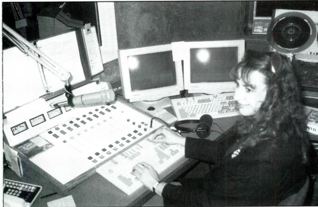
Above. Rebecca Ottun staffs the control room at KJIL-FM/Meade, Kan. The station uses the TM Century Ultimate Digital Studio for music play and the Digital Commercial System from Computer Concepts to replace cart machines.
