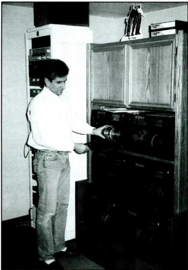
Mike Luskey, director of operations for KJIL-FM/Meade, Kan., inserts a new compact disc in the Ultimate Digital System in the control room.
