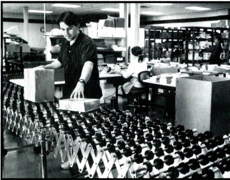
This conveyor speeds up order fulfillment. A larger shipping and mailing area is now on the same level as the shipping docks, eliminating the need for elevators.
