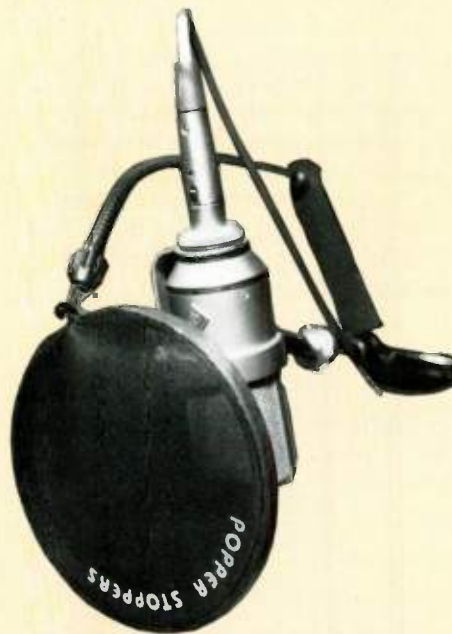
A commercially available blast filter in front of a Neumann TLM-170 microphone.
