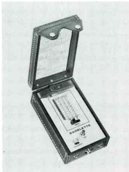
Bar Graph dB read-out, allowing the installer to operate the meter in the carrying case.
