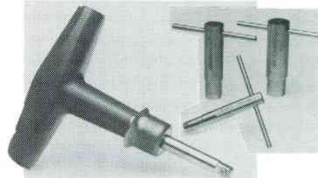
allows the loosening of bolts with easy one hand operation.
