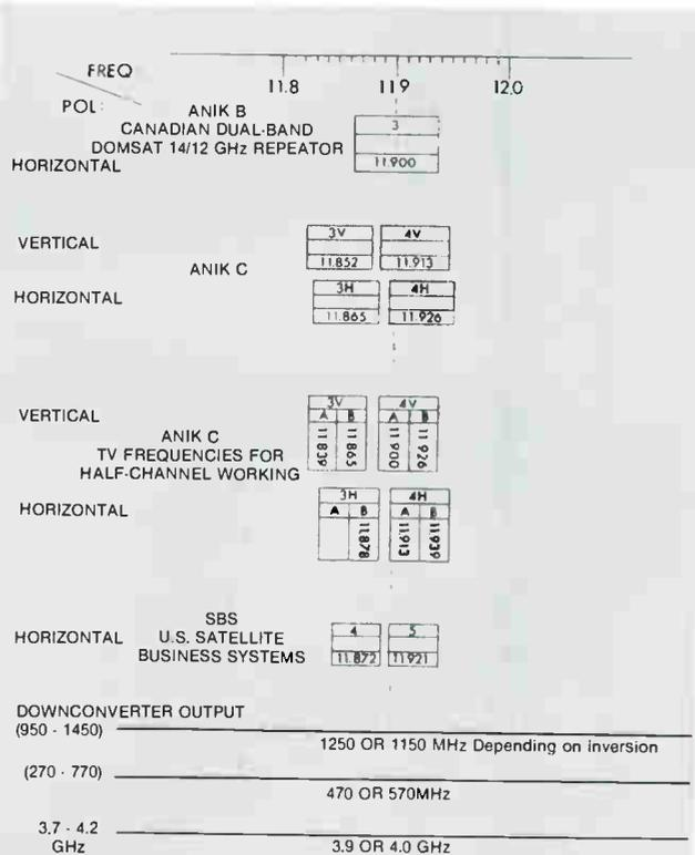
Figure C: Channel Frequency Assignments For 12GHz Satellites
