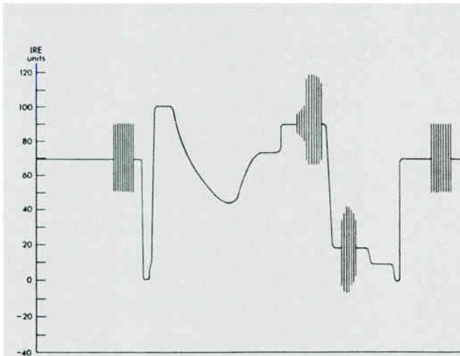
Figure F: Suppressed Sync Video Signal
