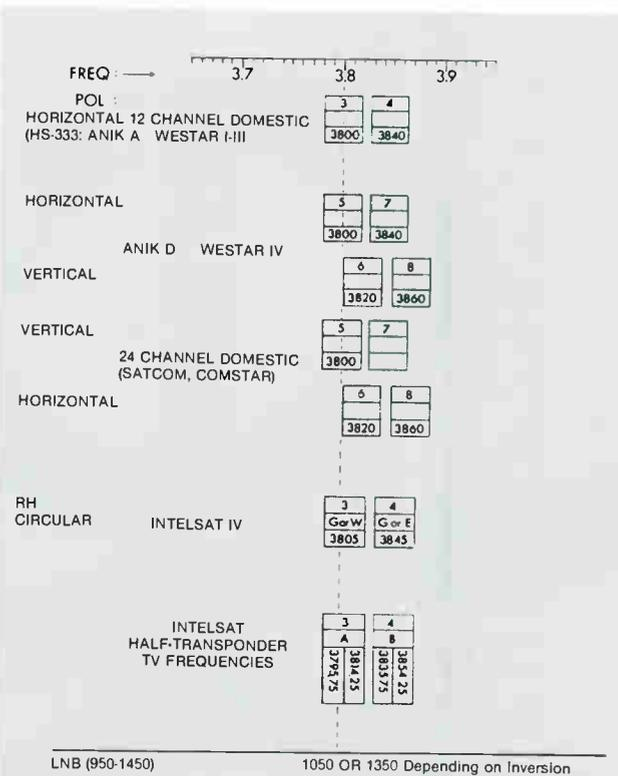
Figure B: Channel Frequency Assignments For 4GHz Satellites
