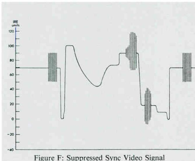
Figure F: Suppressed Sync Video Signal
