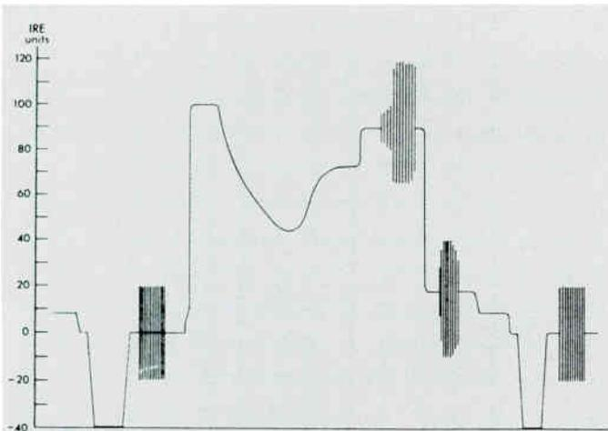
Figure D: NTSC Video Signal
