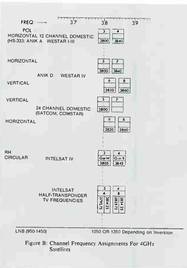
Figure B: Channel Frequency Assignments For 4GHz Satellites
