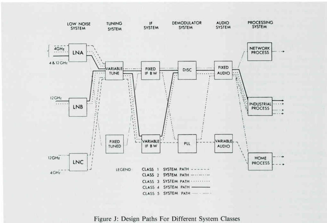
Figure J: Design Paths For Different System Classes
