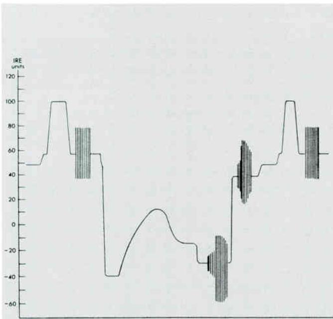
Figure E: Inverted Video Signal
