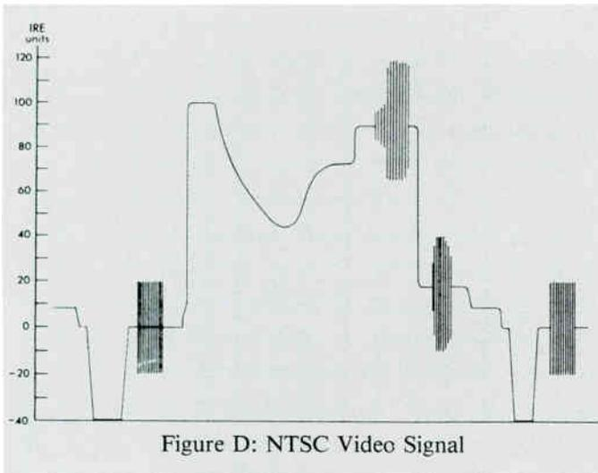
Figure D: NTSC Video Signal
