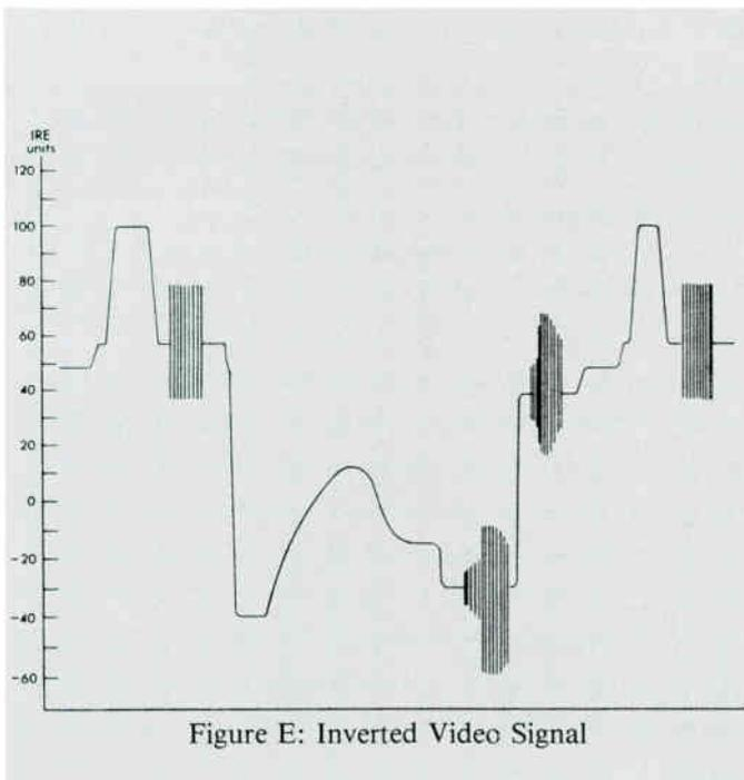
Figure E: Inverted Video Signal
