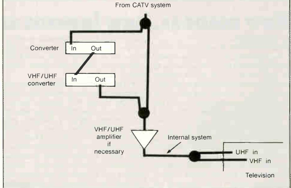
and sent through the existing loop. At the set the cable was split and connected to both the VHF and UHF terminals.
