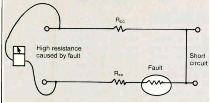
However, if we look at the same length of drop wire from a DC point of view, we are looking at two resistors—the resistance of the center conductor ( $R_{cc}$ ) and the resistance of the sheath ( $R_{sc}$ ). This can be drawn as a simple resistor diagram (Figure 2).
