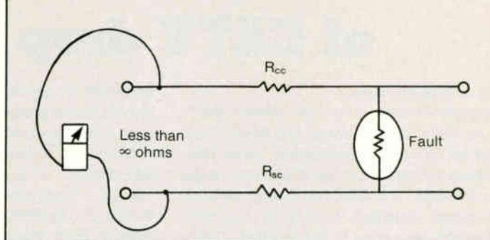
( $\infty$ ) ohms resistance between the two conductors measured using an ohmmeter set on its highest resistance scale. In other words, the ohmmeter movement will not move or, in the case of a digital ohmmeter, the digits will flash 999, 111 or something exhibiting infinity (Figure 4). That is the case of a good drop wire. What about the faulty drop wire?
