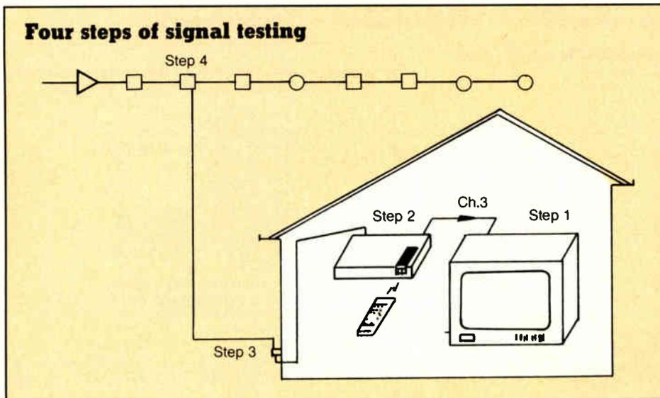
to the TV set. Remember that we are looking for about +3 dBmV and that anything less than 0 dBmV could be causing your problem. The next point of measurement is at the converter input, where a converter is being used (Step 2) to ensure that it is not a converter problem. Again, we would like to have +3 dBmV at the converter input.
