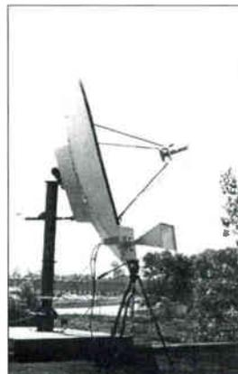
**Set up for suppressing wideband (digital) TI on 4 GHz TVRO.**
