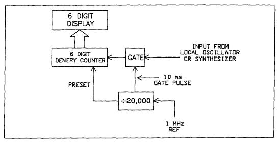
Figure 14. Basic frequency counter.
