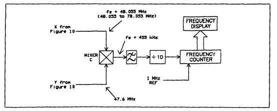
Figure 15. FC arrangement for partial synthesizer of Figure 10.
