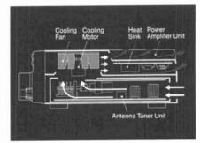
DFCS (Duct Flow Cooling System): This unique system allows 100% duty cycle on FM and RTTY for up to 30 minutes of continuous transmission.
