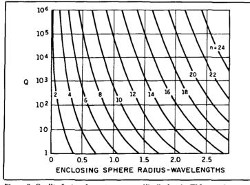
Figure 9. Quality factors for antennas, specifically for the TMmn and TEmn propagation modes, as a function of the enclosing sphere radius in wavelengths. The quality factor is the ratio of stored to dissipated energy, essentially the common Q. See text for usage. After Harrington and Chu.
