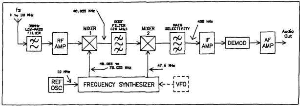
Figure 9. Up-conversion receiver, preferred configuration.
