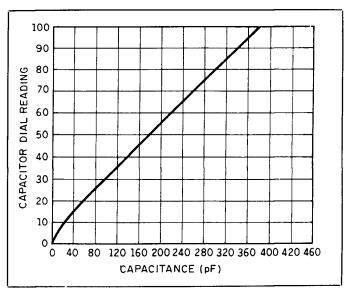
Figure 5. Capacitor dial calibration curve.
