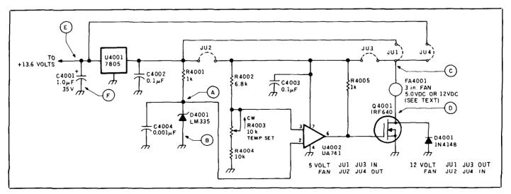
Figure 4. Fan control circuit.
