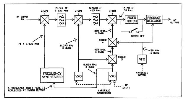
Figure 19. Variable bandwidth, IF shift, and tuneable notch.
