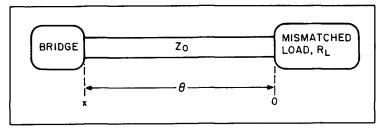
Figure 6. Transmission-line representation for admittance or impedance measurements. The dashed line at 0 is the point at which the load is connected. The reference point x, where the input impedance is determined, is at a distance  $\theta$ , measured in electrical degrees, from the 0 reference line. For this measurement, load R<sub>L</sub> cannot be equal to Z<sub>0</sub>; it must be a mismatched load.
