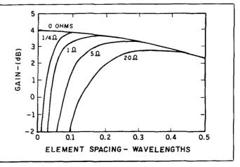
Figure 4. Effect of element resistance on the overall gain of a 8JK array. Compare to *Figure 2*. Calculation is based on resistance being distributed along the antenna length. Usual calculation assumes that the resistance is concentrated at the center of the element.
