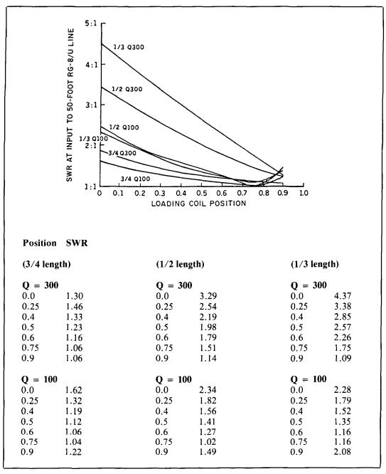
Figure 6. SWR at input end of 50-foot RG-8/U coax used in text example at 7.15 MHz.
