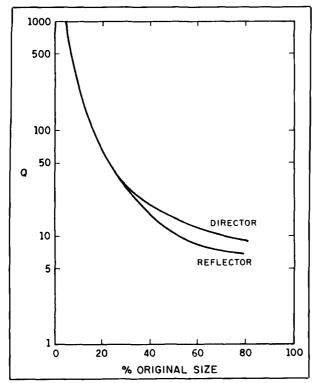
Figure 12. Quality factor for a two-element Yagi, assuming that original size is 0.5 wavelength spacing, and that spacing is gradually decreased. This is the drive point Q, the ratio of drive reactance to drive resistance, and is not the same as that shown in *Figure 9*.
