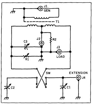
Figure 2. Practical admittance bridge circuit.
