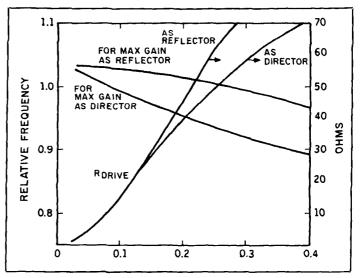
Figure 11. Effect of element spacing of a two-element Yagi, both elements 0.5 wavelengths long. Gain increases slowly as spacing is reduced, but drive resistance decreases rapidly, becoming zero at very close spacing.
