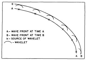
Figure 1. Illustrating Huygens Principle, where a new wave front is created by the envelope of wavelets originating from each point on the original front.
