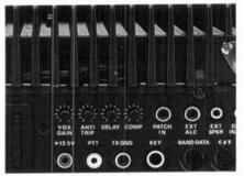
Rear Panel: Seldom used controls are located on rear panel allowing clean uncluttered front panel design.
