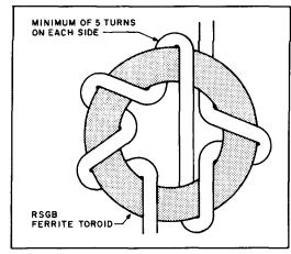
Figure 1. Method of winding choke balun.
