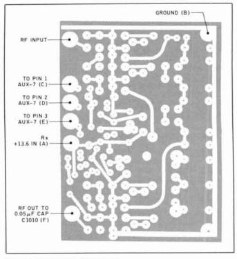
Figure 5. Front-end card foil layout.
