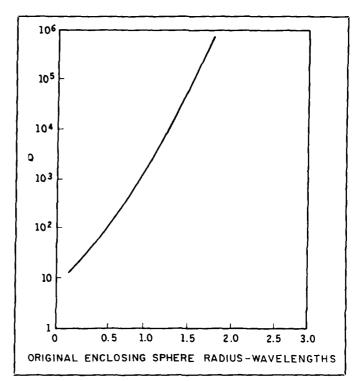
Figure 10. Quality factors for antennas reduced 2:1 in size, as a function of the original enclosing sphere radius. Note that reducing the size of large antennas means that they rapidly become narrow-band devices.
