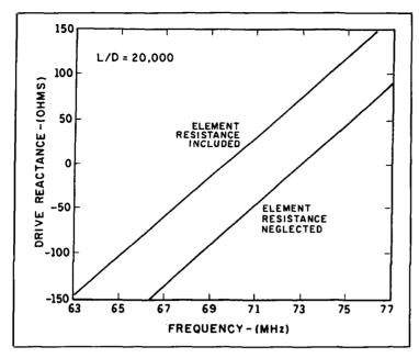
Figure 8. Change in reactance with frequency for a fine wire element with element resistance neglected and considered. The resonant frequency is affected, with a small change in reactance slope. The effects in *Figures 5* through 8 are commonly neglected in antenna textbooks.
