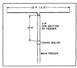
Figure 2. A 14.2-MHz CFR half-wave dipole.
