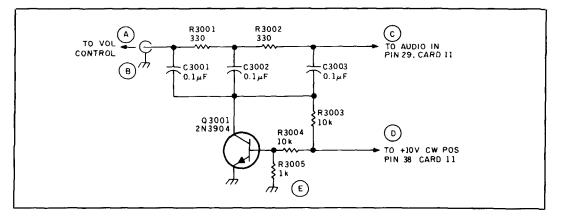
Figure 2. Audio filter circuit.
