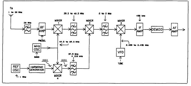
Figure 8. Wadley loop receiver-Racal RA17.
