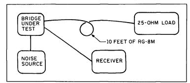
Figure 7. Test setup used to evaluate admittance bridge accuracy.
