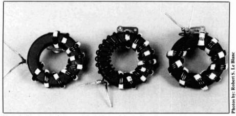
Photo A. The three basic forms of the 1:1 balun: left, the Guanella (current) balun; center, the Ruthroff balun; and right, the trifilar (voltage) balun.
