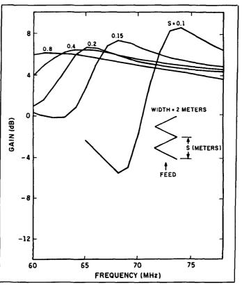
Figure 20. Gain away from the feed point for a zig-zag antenna of several elements and spacings. Note that the span is kept constant, which means that the element length increases as end spacing increases.
