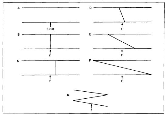
Figure 16. Schematic of a family of direct-coupled antennas. A, no coupling; B, neutral coupling; C, positive coupling; D, E, F, negative coupling of varying magnitudes; G, a variation of F. See text for concept.
