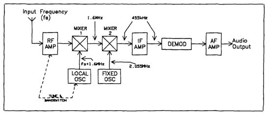
Figure 4. Double-conversion superhet, variable first LO.
