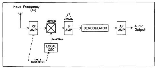
Figure 2. Single-conversion superhet receiver.
