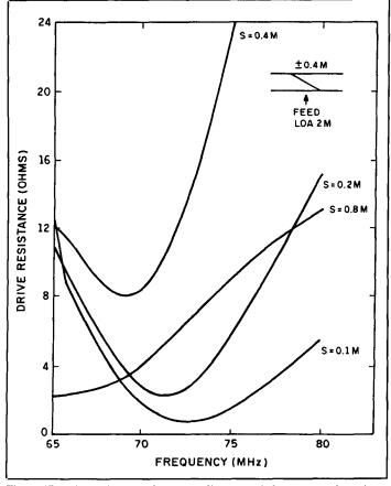
Figure 17. Drive resistance of negative direct-coupled antennas of varying spacing. Both elements identical in size.
