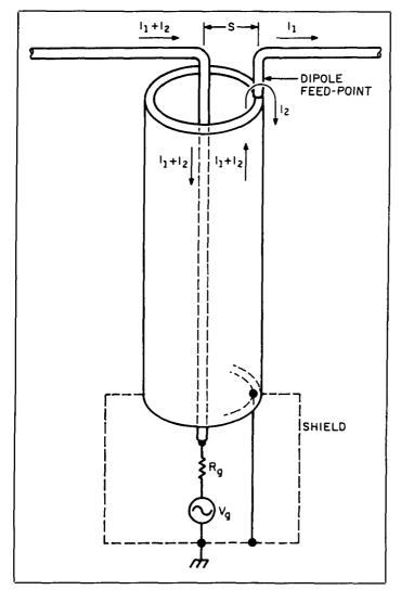
Figure 3. An illustration of the various currents at the feed-point of a dipole. I1 is the dipole current and I2, the inverted L current.
