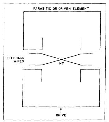
Figure 15. Principle of "antenna neutralization" as developed by Moxon, G6XN. Two dipoles are shortened by folding the element ends, resulting in over-coupling and low drive resistance. The coupling is opposed or "neutralized" by introducing a pair of short elements that couple small out-of-phase components into the wire ends. See text.
