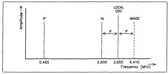
Figure 3. Spectrum of receiver signals.
