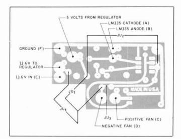
Figure 8. Fan control foil layout.
