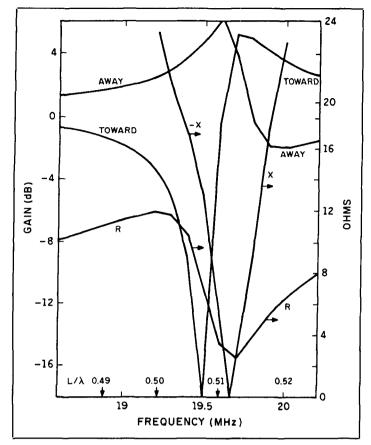
Figure 14. Swept frequency performance of a close-spaced two-element open-loop quad. Elements are of copper tubing and identical in length. The marked change in drive resistance is characteristic of close-spaced arrays, and is not normally found at wide spacing. This antenna performs quite well in a small space.
