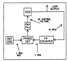
Figure 11. PLL with programmable divider.
