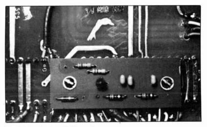
Photo I. Mounting the audio filter card.
