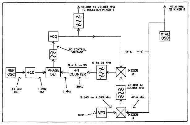
Figure 12. Phase locked partial frequency synthesizer.
