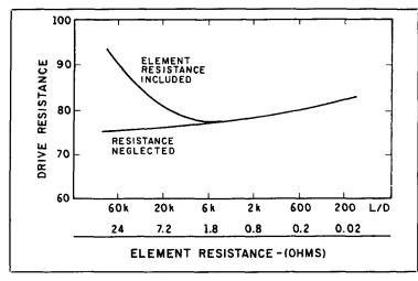
Figure 6. As for *Figure 5*, but showing the effect of element size on drive point resistance. See text.
