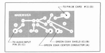
Figure 7. Audio filter foil layout.
