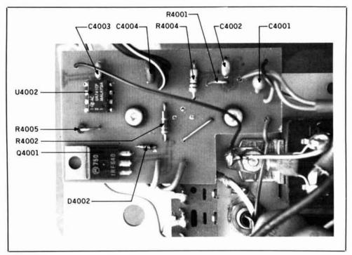
Photo D. Fan control layout.
