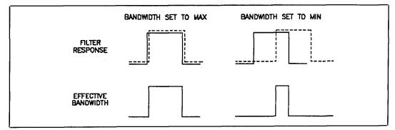
Figure 18. Variable bandwidth response.
