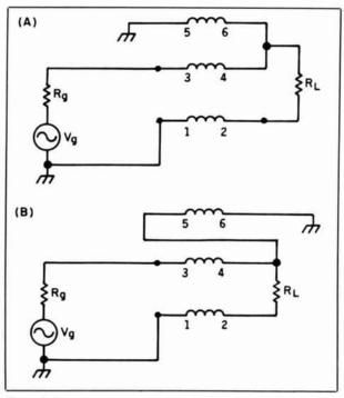
Figure 2. The schematic diagrams of the two basic forms of the three-conductor 1:1 balun. (A) The Ruthroff balun. (B) The voltage balun (originator unknown).
