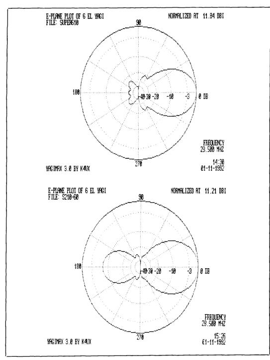
Figure 13. Effect of shrinking the boom length of a six-element Yagi to 60 percent of its original size, and retuning some elements. A is for the original size, B for the reduced size. Further element adjustment can increase the smaller antenna gain. See text.
