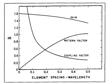
Figure 2. Theoretical gain of a two-element end-fire array, or 8JK antenna, showing the pattern factor, the coupling factor, and the overall gain. Element resistance is neglected.
