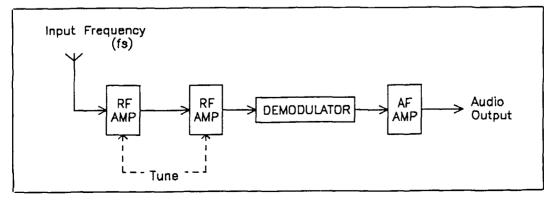
Figure 1. The TRF receiver.
