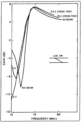
Figure 18. As *Figure 17*, but for gain away from the parasitic element (reflector action). Over much of the frequency range, this mode gives the best forward gain.
