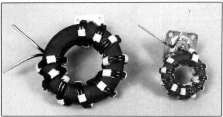
Photo C. High-power (on the left) and low-power (on the right) versions of the coiled-wire (transformer-type) Guanella 1:1 balun. These baluns are also known as current or choke baluns.
