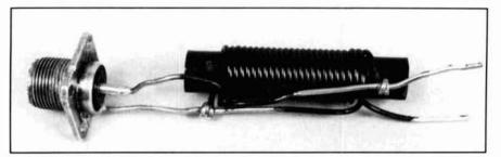
Photo B. A typical 1:1 rod-type voltage balun (W2AU).
