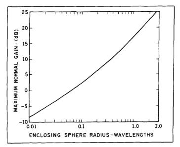
Figure 3. Maximum normal gain of an antenna from Harrington and Chu as a function of the radius of the sphere just enclosing the antenna. If the gain is less than the curve value, the antenna is in the normal (gain) range, if greater, in the supergain regime.
