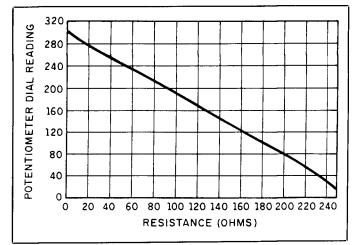
Figure 4. Potentiometer dial calibration curve.
