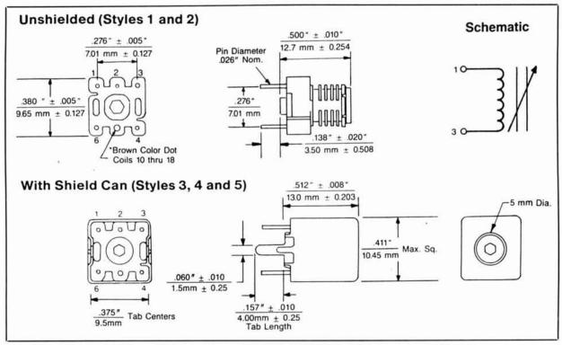
Figure 1. Slotted bobbin enhances temperature stability and supports electromagnetic shielding ring. Standard- sized 10-mm can provides electrostatic shield. (Courtesy of Coilcraft.)
