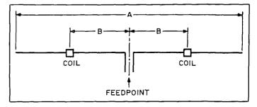
Figure 1. Dimensions relating to shortened dipole.
