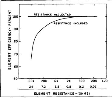
Figure 5. Calculated efficiency of a dipole as a function of element size. Based on a 2-meter long element at 75 MHz. Curve is approximately correct for any dipole of the same length/diameter ratio, but the exact value varies due to skin effect on element resistance.
