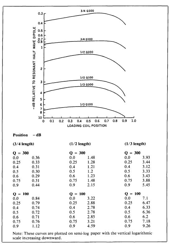
Figure 4. Signal strength of shortened antennas relative to full-size half wave resonant dipole as function of coil position.
