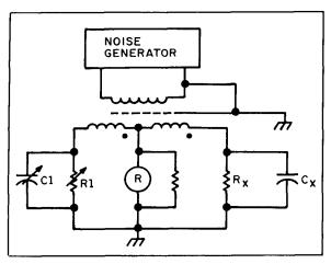
Figure 1. Basic admittance bridge circuit.
