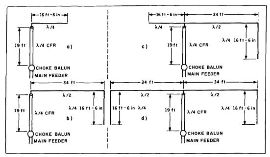
Figure 3. CFR antennas: (A) isotrophic, (B) half square (C) half square, (D) bobtail.
