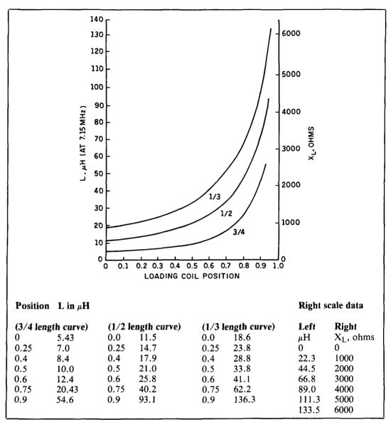
Figure 2. Inductance and reactance of loading coils required (at 7.15 MHz in text example) for dipoles shortened to 3/4, 1/2, and 1/3 times length of full-size *resonant* half wave dipole as a function of coil position (decimal fraction of B/(A/2). If reactance is used (right scale) curves in *Figures 2, 3,* and 4 are frequency independent.
