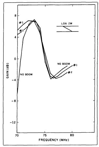
Figure 19. As Figure 17, but for gain toward the parasitic element (director action).
