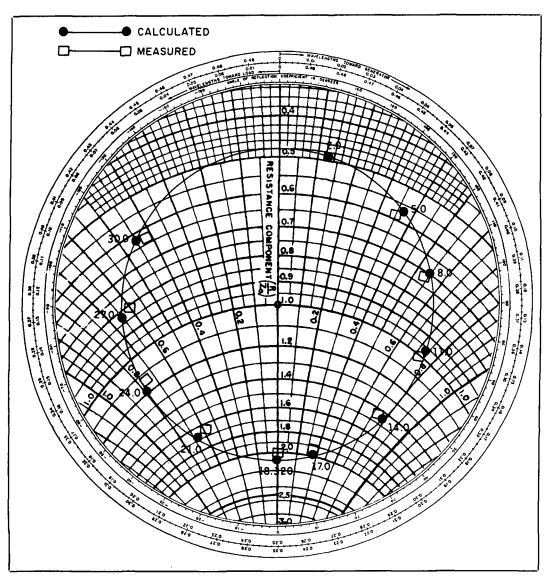
Figure 8. Normalized Smith chart representing measured and calculated impedance points.
