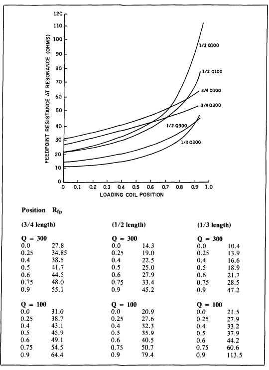
Figure 5. Feedpoint resistance at resonance.
