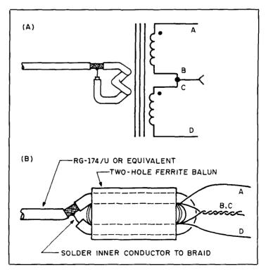
Figure 3. Details of admittance bridge transformer. (a) Circuit diagram. (b) Method of winding transformer.
