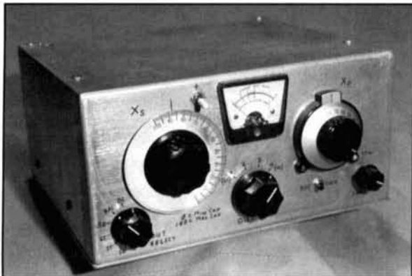
Photo A. The IBZ Coupler mounted in bottom-opening cabinet.
