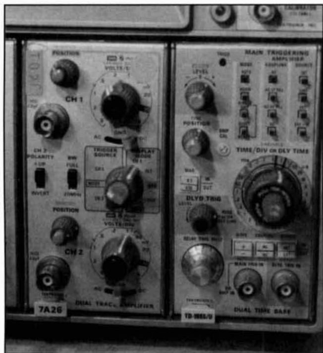
Photo C. Note that all functions and settings are included on the front panel of a traditional analog scope.
