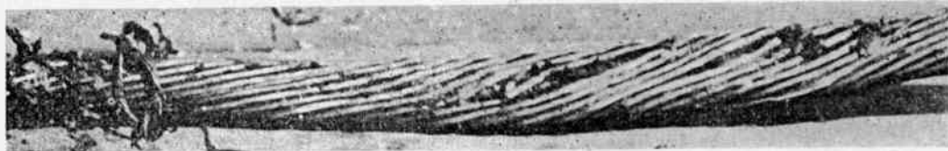
The first damage. The copper conductor is showing between the displaced iron armor wires
