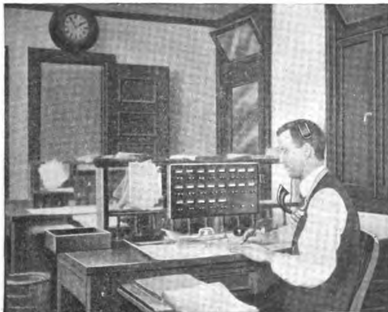
DISPATCHER USING CHEST TRANSMITTER AND HEAD RECEIVER.
