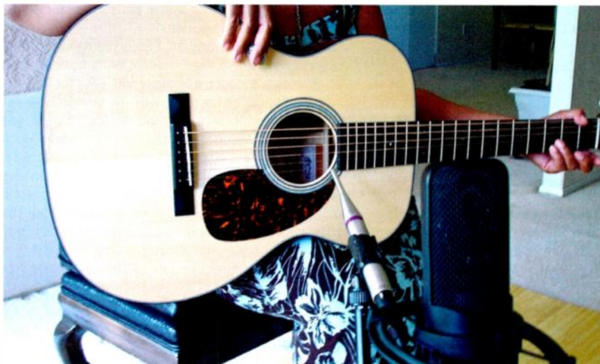
A two mic set-up, with the close mic at the spot where the neck meets the sound hole.
