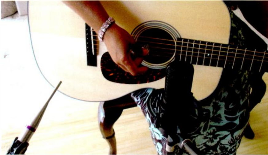
You can capture a very balanced tone by using a large diaphragm condenser mic close to the soundhole and a second mic pointing at the bridge.
