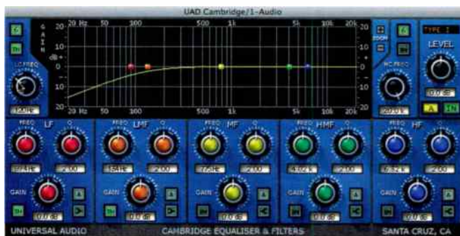
The hi-pass filter on this UAD Cambridge EQ is set to remove unneeded low end from a track that was competing with the bass.
