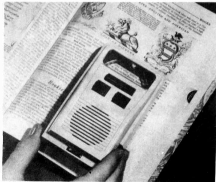
The Microsonics Corporation has recently introduced a compact audio/visual system capable of bringing sound to the printed page. The system utilizes a handheld microphonograph that plays a transparent audio disc mounted on printed material to provide up to 90 seconds of audio information.
