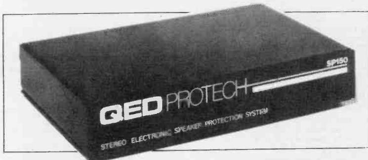
**QED Audio Products'** Protech SP150 is a handy companion to loudspeaker drive units — it protects them from overloading. Deriving its power from the signal source, the SP150 constantly monitors the signal to the speakers. In the event of an overload, a time delay is triggered. If the level doesn't drop to within a lower range, a relay cuts the power to a safe measurement.
