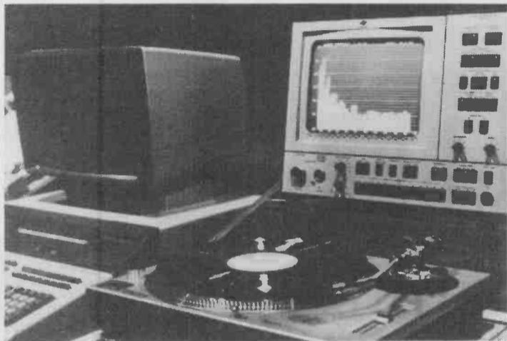
One of the most frequent consumer complaints about phonograph records is their pressing quality. Now, one record industry thermoplastics supplier has devised a computerized noise analyzer that can trace the origins of sound discrepancies on recorded discs.
