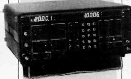
**Amber Electro Design** has introduced the model 5500, a programmable audio measurement system. It can measure virtually every performance parameter of audio systems and components, including gain, frequency response, output power, weighted and unweighted noise, crosstalk, total harmonic distortion, and intermodulation distortion.
