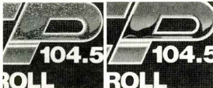
After the test, the equivalent of a year in the weather, note the peeling, fading and cracking in the "label" type product (left). The Communication Graphics decal (right) still looks great.
