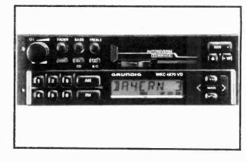
Grundig RDS-equipped receiver displaying West German Bayern 3 network station
