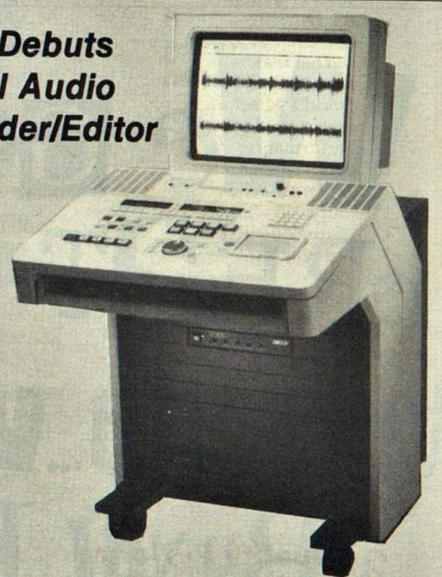
Otari Corp.'s professional digital audio recorder/editor is a fully integrated and configured "plug in and use" production console that incorporates support software from Menlo Park, CA-based Digidesign.
