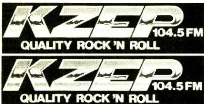
In a General Motors developed test, stickers are aged the equivalent of one year's exposure to the elements. The top sticker was produced by Communication Graphics, the bottom by another company. As you can see, they appear identical "off-the-press."
