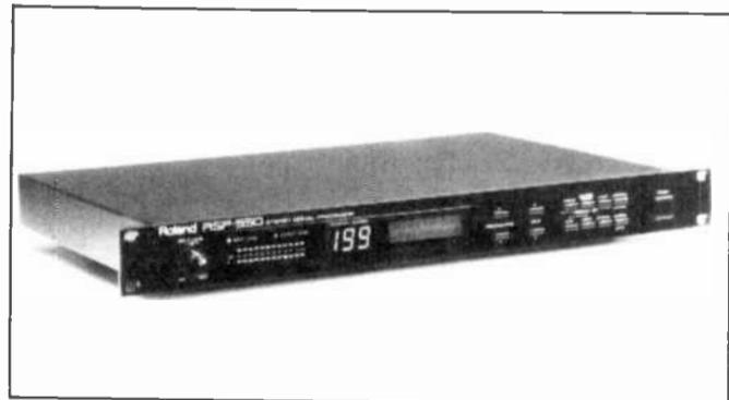
Roland's new "RSP-550" stereo signal processor contains a number of effects, including reverb, multitap delay, enhancer, equalization, flanging, phasing, chorus, rotating speaker, and vocoder.
