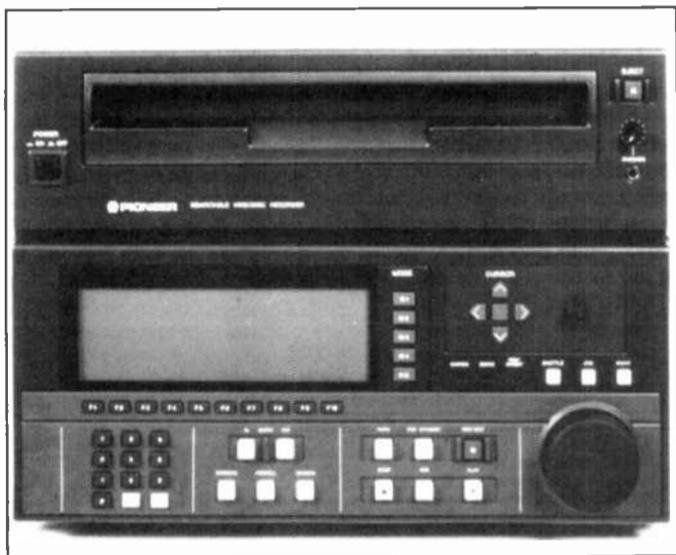
**R**ecording technology has taken a leap forward with the recent introduction of Pioneer's "VDR-V1000 LaserRecorder," a rewritable videodisc recorder that can erase and rewrite information stored on videodiscs up to one million times.
