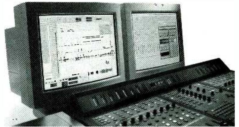
A full-blown Pro Tools system, with the Pro Control console in the foreground.
