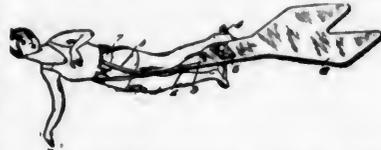
A swimming appliance, including a web, foot rests extending in opposite directions from the web, a tail portion extending from the web and adapted to be flexed by the foot rests, and means for attaching the web to the user.
