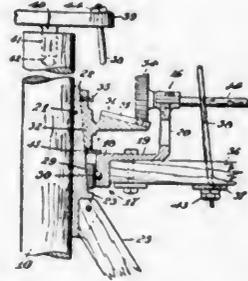
In a merry-go-round, a standard, an annular-toothed rack encircling said standard, a superstructure, revoluble around said standard, a rotary shaft carried by said superstructure, a pinion on said shaft meshing with said rack, a rotary plate journaled on said standard above said rack, and adjustable depending rods suspending said superstructure from said plate.
