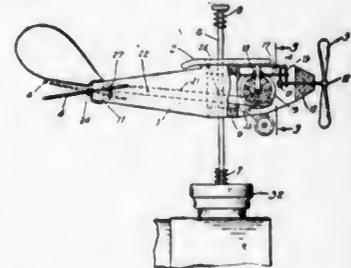
A toy airplane of the class described, in combination with a fuselage, adapted to rise and fall on a pole passing thru said fuselage; a propeller, adapted to turn by the velocity of air passing therethru; an elevator, a power of transmission means connected between the said propeller and elevator, and a rudder secured to the upper-rear end of the said fuselage, as set forth.
