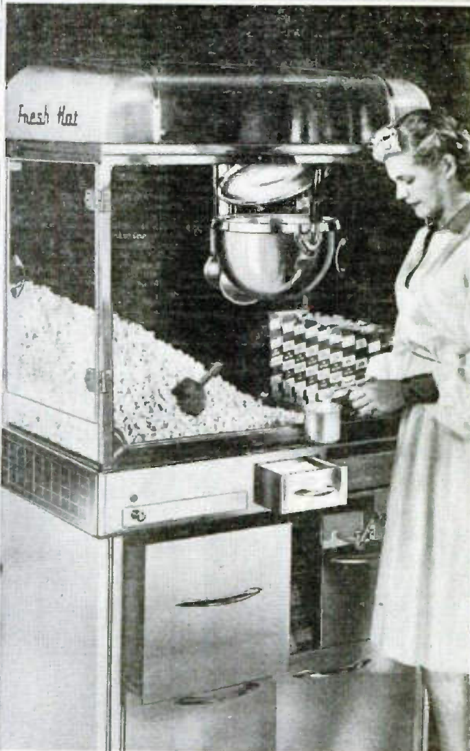
REMOVABLE HOOD permits adjustments in top of machine... Electric shock prevented by circuit breaker operating automatically as top is removed.
