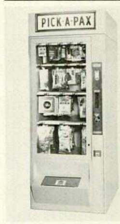
vender carries up to 15 different items at up to 12 different prices, ranging from 5 cents to \$1.50. Items are suspended by plastic tabs on a "snatch" auger. Unit has a six-second maximum vending cycle, has a National SCS changer, safety plate glass front and measures 70 by 31 by 31 inches.
