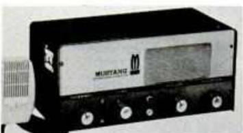
The Mustang, a citizen's band transceiver, has been introduced by Metrotek Electronics, a subsidiary of Regency Electronics. The unit has six crystal-controlled transmit channels and may be tuned to receive all 23 channels. It transmits on any six of the 23 available CB channels. Plug-in crystals, mounted on the chassis, can be changed to provide any desired frequency. Power output is 3.0 watts, minimum. A high impedance ce-
