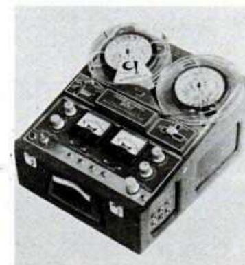
A professional-style control panel of slant design is the chief new feature of the Model 800 three-speed, four-track stereo tape recorder manufactured by Freeman Electronics. The unit has built-in speakers, dual VU meters, tone and volume controls for each channel, three stereophonic output jacks, radio-phono and FM multiplex input jacks and jockey stick function control. The suggested price is \$299.50.
