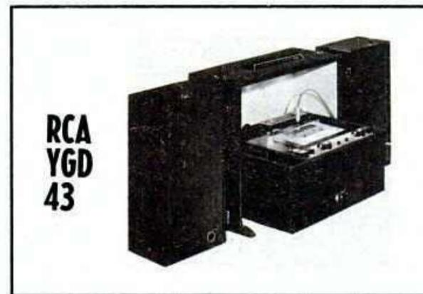
Tape speeds —  $1\frac{7}{8}$  and  $3\frac{3}{4}$  ips. Heads — four. Motors — one. Record — 4-track mono and 4-track stereo. Playback — 4-track mono and 4-track record. Frequency response — 50-15,000 cps. Indicator — meter. Weight —
