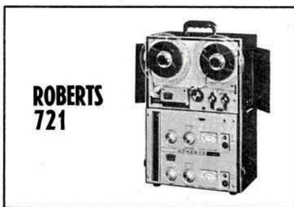
Tape speeds —  $3\frac{3}{4}$  and  $7\frac{1}{2}$  (15 optional) ips. Heads — two. Motors — one. Record — 4-track mono and 4-track stereo. Playback — 4-track mono and 4-track stereo. Frequency response — 40-17,000 cps. Indicators — 2 meters. Weight — 49 lb. Other features — self-contained carrying case; 2 microphone and 2 radio-phono inputs; 2 preamp, 4 headphone, 2 extension speaker, 2 sound head outputs; sound-with-sound; sound-on-sound; monitoring; automatic shutoff. Price — \$359.95.
