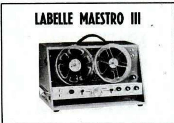
**Tape speeds** —  $3\frac{3}{4}$  and  $7\frac{1}{2}$  ips. **Heads** — one. **Motors** — one. **Record** — 2-track mono. **Playback** — 2-track mono. **Frequency response** — 50-15,000 cps. **Indicator** — 2 neon lamps. **Weight** — 28 lb. **Other features** — self-contained carrying case; microphone and radio-phono inputs; external speaker output; slide projector sync; pulse; speaker built into carrying case cover. **Price** — \$375.
