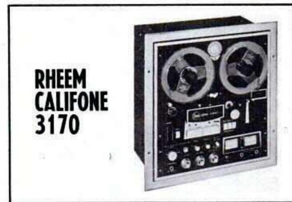
Tape speeds —  $3\frac{1}{2}$  and  $7\frac{1}{2}$  (15 optional) ips. Heads — three. Motors — three. Record — 4-track mono and 4-track stereo. Playback — 4-track mono and 4-track stereo. Frequency response — 40-18,000 cps. Indicators — 2 meters. Weight — 54 lb. Other features — deck, with preamps only. 2 microphone and 2 radio-phono inputs; 2 preamp, headphone outputs. Automatic shutoff; sound-on-sound; sound-
