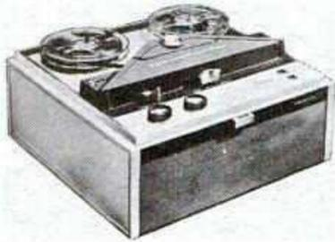
**Tape speeds** —  $3\frac{3}{4}$  and  $7\frac{1}{2}$  ips. **Heads** — two. **Motors** — one. **Record** — 2-track mono. **Playback** — 2-track mono. **Frequency response** — 150-12,000 cps. **Meter** — none. **Weight** — 19 lb. **Other features** — self-contained carrying case; microphone input; preamp headphone outputs; slide sync provision; built-in speaker. **Price** — \$109.95.
