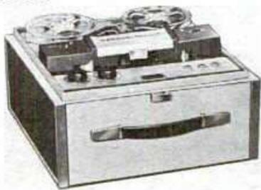
**Tape speeds** —  $1\frac{7}{8}$ ,  $3\frac{3}{4}$  and  $7\frac{1}{2}$  ips. **Heads** — two. **Motors** — one. **Record** — 4-track mono. **Playback** — 4-track mono. **Frequency response** — 100-15,000 cps. **Indicator** — meter. **Weight** — 21 lb. **Other features** — self-contained carrying case; microphone and radio-phono inputs; preamp and external speaker outputs; 2 built-in speakers. **Price** — \$159.95.
