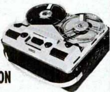
Tape speeds — 1 7/8, 3 3/4 and 7 1/2 ips. Heads — two. Motors — one. Record — 4-track mono and 4-track stereo. Playback — 4-track mono and 4-track stereo. Frequency response — 30-18,000 cps. Indicator — electric eye. Weight — 29 lb. Other features — self-contained carrying case; 2 microphone and 4 radio-phono inputs; 2 preamp, 2 external speaker and 2 headphone outputs; sound-on-sound; sound-with-sound; one speaker built-in, one in
