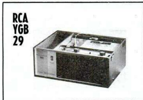
Tape speeds —  $1\frac{7}{8}$  and  $3\frac{3}{4}$  ips. Heads — four. Motors — one. Record — 4-track mono. Playback — 4-track mono. Frequency response — 50-15,000 cps. Indicator — meter. Weight — not available. Other features — cartridge machine; self-contained carrying case; microphone and radio-phono inputs; preamp outputs; and earphone; remote control mike; built-in speaker. Price — \$129.95.
