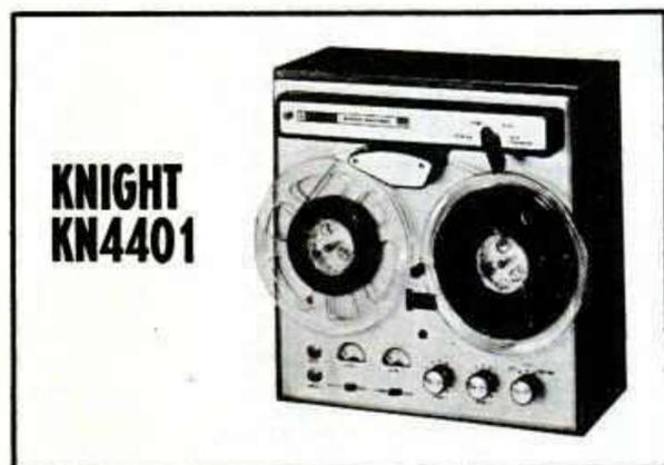
**Tape speeds** —  $3\frac{3}{4}$  and  $7\frac{1}{2}$  ips. **Heads** — two. **Motors** — one. **Record** — 4-track mono and 4-track stereo. **Playback** — 4-track mono and 4-track stereo. **Frequency response** — 50-15,000 cps. **Indicators** — 2 meters. **Weight** — 31 lb. **Other features** — deck with preamps only; 2 microphone and 2 radio-phono inputs; 2 preamp, 2 tape head outputs. **Price** — \$169.95.
