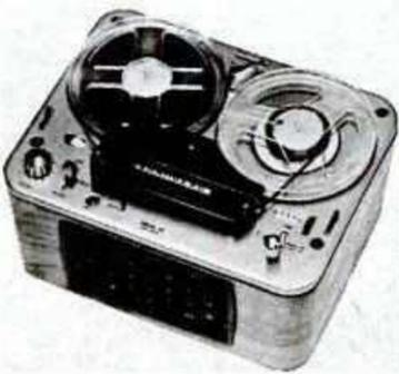
Tape speeds — 1 7/8, 3 3/4 and 7 1/2 ips. Heads — two. Motors — one. Record — 2-track mono. Playback — 2-track mono. Frequency response — 40-16,000 cps. Indicator — electric eye. Weight — 22 lb. Other features — microphone and radio-phono inputs; speaker output; remote control; built-in speaker. Price — \$344.50; without remote control and remote control foot pedal, \$269.50.
