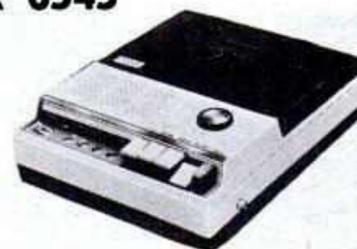
Tape speeds —  $1\frac{7}{8}$ ,  $3\frac{3}{4}$  ips. Heads — two. Motors — one. Record — 2-track mono. Playback — 2-track mono. Frequency response — 150-7000 cps. Indicator — meter. Weight — 6 lb. Other features — powered by 6 C-cell batteries; remote control microphone and radio-phono inputs; earphone output; built-in speaker. Price — \$109.95.
