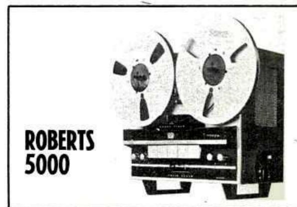
Tape speeds —  $3\frac{3}{4}$  and  $7\frac{1}{2}$  (15 optional) ips. Heads — three. Motors — three. Record — 4-track mono and 4-track stereo. Playback — full, 2- and 4-track mono and 2- and 4-track stereo. Frequency response — 30-22,000 cps. Indicators — 2 meters. Weight — not available. Other features — 2 microphone and 2 radio-phono inputs; 2 preamp, 2 external speaker, headphone outputs; cross field head; sound-on-sound; all transistor; 2 built-in speakers. Price — \$699.95.
