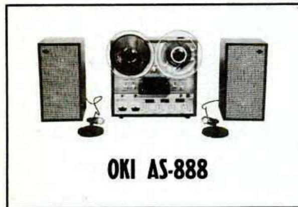
Tape speeds —  $3\frac{3}{4}$  and  $7\frac{1}{2}$  ips. Heads — three. Motor — one. Record — 4-track mono and 4-track stereo. Playback — 4-track mono and 4-track stereo. Frequency response — 40-18,000 cps. Indicators — 2 meters. Weight — not available. Other features — walnut base; 2 microphone, 2 radio-phono, and 2 auxiliary inputs; 2 preamp and 2 speaker outputs; sound-on-sound; sound-with-sound; 2 bookshelf speakers in walnut enclosures. Price — \$489.85.
