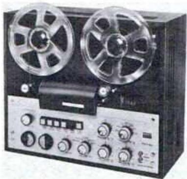
Tape speeds —  $3\frac{3}{4}$  and  $7\frac{1}{2}$  ips. Heads — three. Motors — three. Record — 4-track mono and 4-track stereo. Playback — 2 and 4-track mono and 4-track stereo. Frequency response — 25-18,000 cps. Indicators — 2 meters. Weight — 48 lb. Other features — deck with preamps; 2 microphone and 2 radio-phono inputs; 2 preamplifier and headphone outputs; sound-on-sound. Price — in semi kit form, \$299.95.
