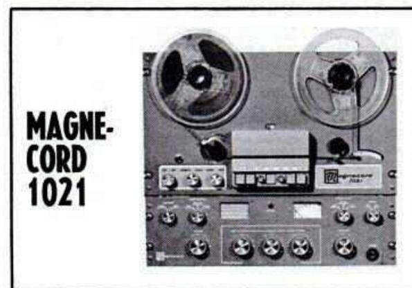
**Tape speeds** —  $3\frac{3}{4}$  and  $7\frac{1}{2}$  ips. **Heads** — three. **Record** — full track mono. **Playback** — full and 2-track mono. **Frequency response** — 45-18,000 cps. **Indicator** — meter. **Weight** — 47 lb. **Other features** — deck, with preamp and monitoring amp; 3 microphone and 1 radio-phono input; preamp, speaker, headphone and sound-on-sound; monitoring speaker. **Price** — \$708.
