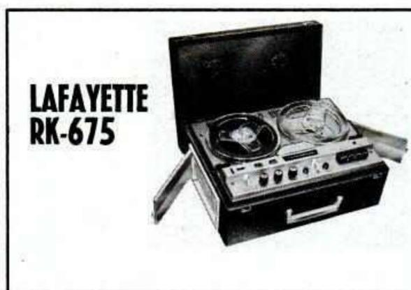
**Tape speeds** —  $3\frac{3}{4}$  and  $7\frac{1}{2}$  isp. **Heads** — two. **Motors** — one. **Record** — 4-track mono and 4-track stereo. **Playback** — 4-track mono and 4-track stereo. **Frequency response** — 40-18,000 cps. **Indicator** — **Weight** — 35 lb. **Other features** — self-contained carrying case; 2 microphone and 2 radio-phono inputs; 2 preamp, 2 external speaker and headphone outputs; 2 built-in speakers. **Price** — \$159.95; Model RK-650, deck with preamps only, \$109.95.
