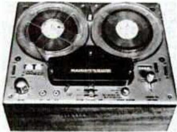
Tape speeds — 1 7/8, 3 3/4 and 7 1/2 ips. Heads — two. Motors — one. Record — 4-track mono and 4-track stereo. Playback — 4-track mono and 4-track stereo. Frequency response 40-16,000 cps. Indicators — electric eye. Weight — 27 lb. Other features — wood base, 2 microphone and 2 radio-phono inputs; 2 preamp and 2 external speaker outputs; sound-on-sound; monitor; 2 built-in speaker. Price — \$449.50.
