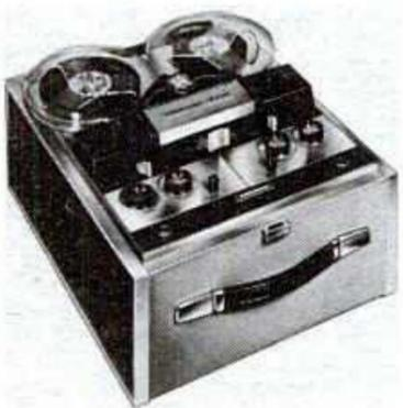
**Tape speeds** —  $3\frac{3}{4}$  and  $7\frac{1}{2}$  ips. **Heads** — one. **Motors** — one. **Record** — 4-track mono and 4-track stereo. **Playback** — 4-track mono and 4-track stereo. **Frequency response** — 50-15,000 cps. **Indicator** — electric eye. **Weight** — 27 lb. **Other features** — self-contained carrying case; 2 microphone inputs; 2 external speaker outputs; 2 built-in speakers. **Price** — \$199.95.
