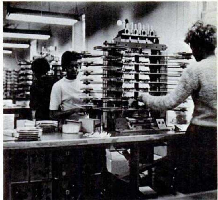
TWO DUBBINGS EMPLOYEES operate one of the firm's new duplicators. The machine enables the operators to duplicate 12 tapes from one master, or a total of 400 eight-track tapes per hour.
