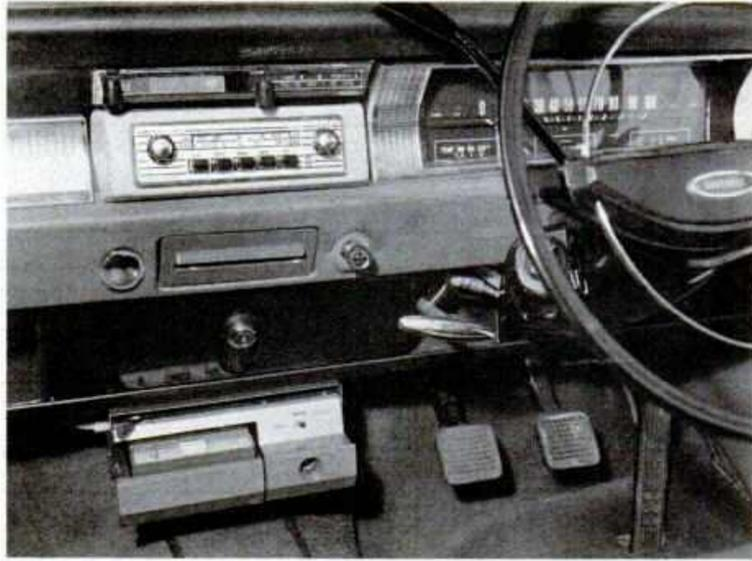
PHILIPS' TAPE CARTRIDGE unit is designed for separate use or in conjunction with the auto radio. The lever-operated tray slides out to take recorder and to facilitate changing of the cassette.
