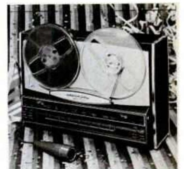
WEBCOR'S NEW HOLIDAY is a two-speed, 4-track stereo/monaural unit that records on all four tracks. Primary feature of this self-contained recorder is its Touch-Tab Control bar. It also has two microphones, two VU meters, twin 5-inch speakers, frequency response from 100 to 15,000 cycles, and automatic shut-off. Suggested retail price is \$199.95.
