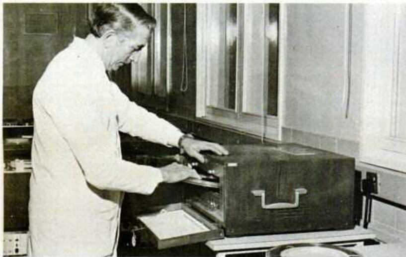
Dubbing operator Harry Munson bulk erases a spool prior to a dubbing run-through. Each spool of tape is erased using the Weircliffe bulk eraser to ensure absolute conformity of magnetic influence prior to the duplicating procedure.
