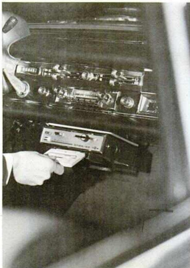
Europe's first authentic car tape recorder, Uher's Snob 100. This is a mono-only record and playback unit which can also be used for domestic applications.
