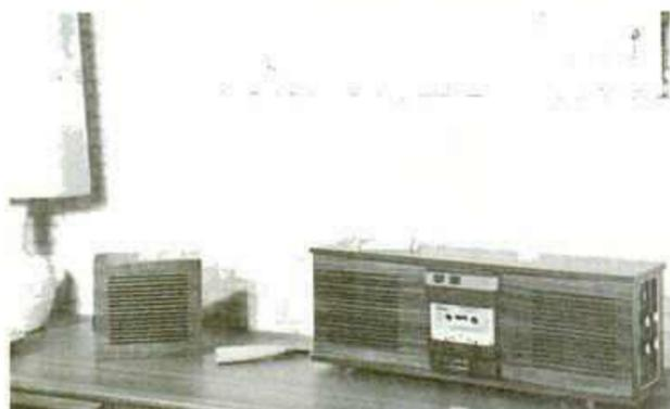
Aimed at the high quality market, Van der Molen's three units were the first British-made stereo machines. A compact/loudspeaker (seen left) can be stowed behind the left-hand grill in the recorder case for mono operation or, as shown, detached for maximum stereo separation.
