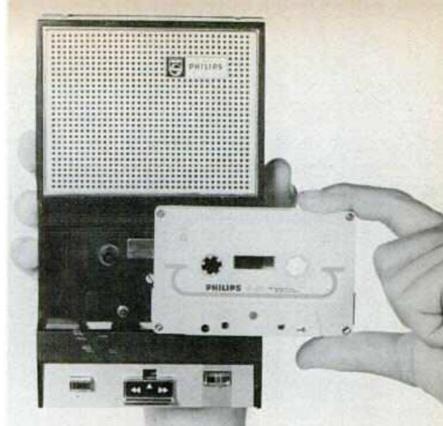
Outstanding feature of the Philips compact cassette is its extreme miniaturization. The portable recorder-playback unit, made in Europe but marketed in the U. S. by Norelco as the Carry-corder, fits easily into a lady's hand.
