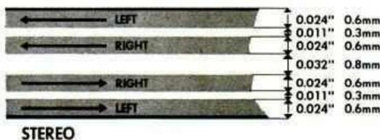
One of the greatest advantages of Philips cassette system is the compatibility of mono and stereo playback and recording.
