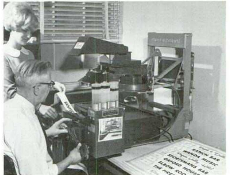
PERMANENT PERSONALIZATION strips for jukeboxes are produced in permanent strips by this photo typositor for use on the Wurlitzer Americana. Wurlitzer makes strips available in 10 type faces and custom art if desired. Special order forms are available through distributors.
