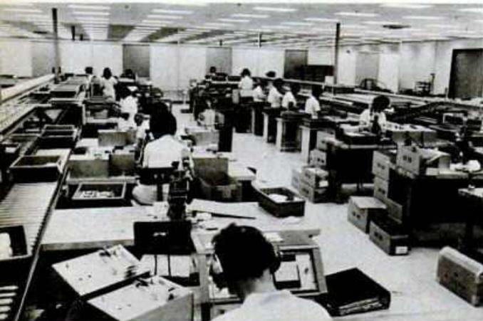
Listening tests used to confirm quality of cartridges after technical quality specifications have been met, giving finished cartridges final audio tests before shipping.
