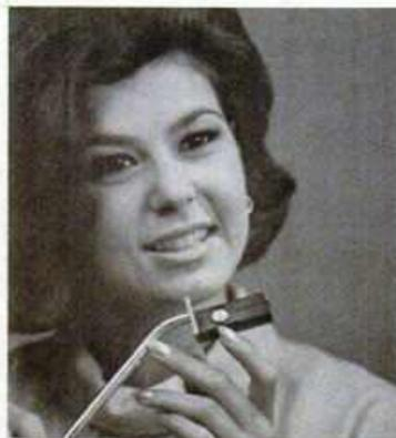
**THE INTEGRATED CIRCUIT** comes to the phonograph in the 1968 RCA Victor line. The IC, under the cap in the tone arm, acts as a pre-amp and is said to reduce the possibility of distortion.
