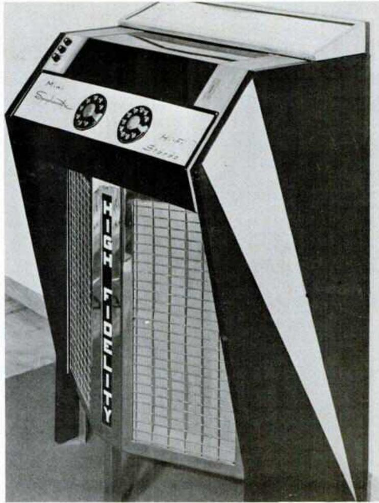
MINI SYMPHOMATIC jukebox designed by John Foufounis, Gerinvex Sa, Switzerland. The extremely simplified unit employs only two small "one-way" electric motors and a pair of start/stop switches. Selections are made from a 40 record magazine utilizing a mechanical principle with two telephone dials. An adaption, the Victor jukebox, is now being produced and sold in Japan.
