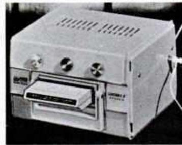
A PORTABLE CARTRIDGE PLAYER, the Cart/able 8, has been introduced by Borg-Warner's spring division. The lightweight, self-contained playback will retail in the \$100 range. Its detachable speakers may be separated up to 18 feet, and a switch converts the player to a transport deck to permit play of 8-track cartridges through other stereo systems. National distribution has begun.
