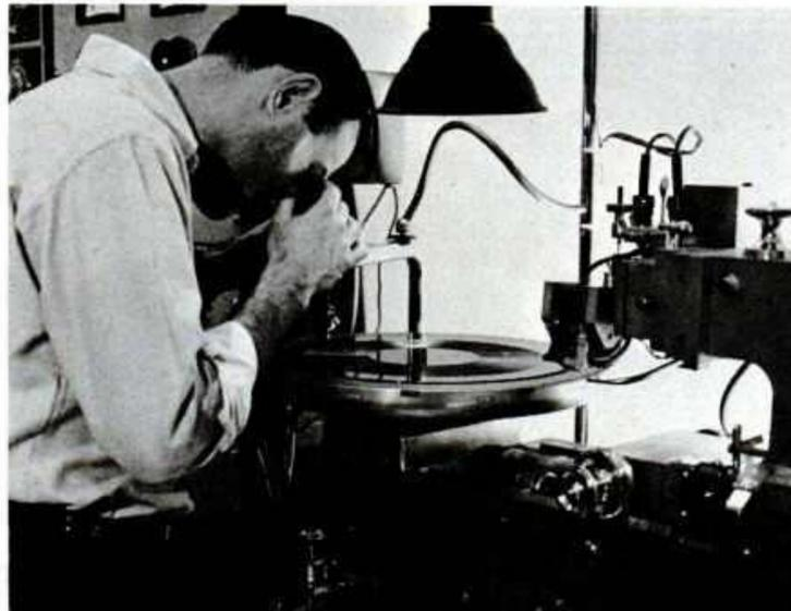
**SOL KESSLER** checks a stereo lacquer before sending it to the plating plant. The lacquer master will be eventually used in the pressing of stereo records.
