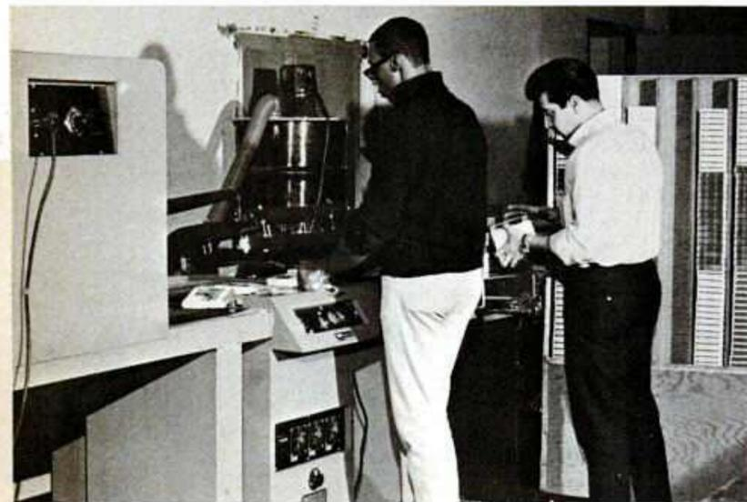
COMPLETED CARtridge is then shrink-wrapped and loaded into boxes for shipment.
