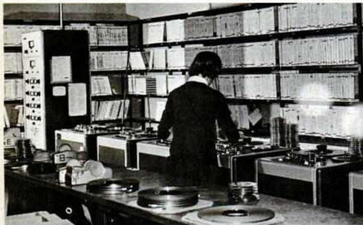
A&B's SECOND DUPLICATION line features a reel-to-reel master controlling 10 slaves for duplication of 4-, 8-track and cassette production. All slaves are equipped with interchangeable plug-in head assemblies, permitting the same equipment to be used for all configurations.
