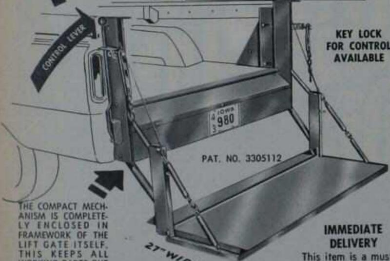
THE COMPACT MECHANISM IS COMPLETELY ENCLOSED IN FRAMEWORK OF THE LIFT GATE ITSELF. THIS KEEPS ALL WORKING PARTS OUT OF WEATHER AND TROUBLE FREE.
