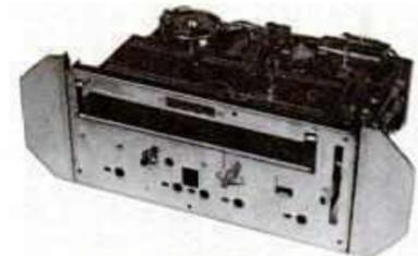
**POWER AMPLIFIER** and drive mechanism of self-contained unit above.
