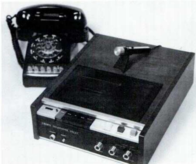
CROWN TELEPHONE VALET, imported and marketed by Industrial Suppliers, answers the phone and receives messages. Model 4400 accepts calls with a pre-recorded 20-second message. The caller's message is then recorded on a voice-activated cassette. After 8 to 15 seconds of silence, the machine is automatically shut off, ready for the next call. The 20-second message is pre-recorded on a continuous loop cartridge. The cassette recorder also doubles as a home player/recorder.
