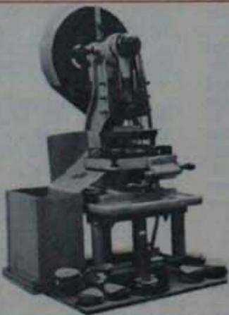
**Fabelex** • Eccentric press 8 tons for cutting of centre and outside  $\varnothing$  7" records
