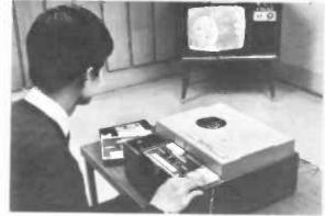
THE SONY Videocassette player is a simple, compact, easy to operate unit. Loading and unloading is a one-hand operation, left. The prerecorded programs are screened through any standard television set, color or black and white, right, by attaching it to the antenna base.
