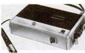
MINIATURE cassette recorder, the RD-406, operates on penlite batteries, 12V car battery, AC, or adapter battery recharger. Weighing 1¾ lbs., Sharp Electronics suggests \$79.95 price.
