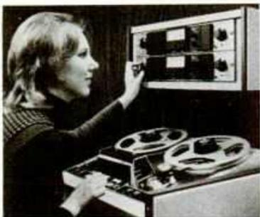
ELECTRO SOUND's ES-505 professional magnetic tape recorder is now being delivered to U.S. and international distributors. The recorder is available in 1/4 in. or 1/2 in. versions, with one to four channels.
