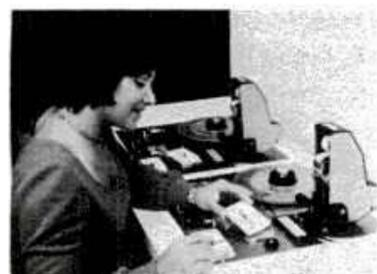
**TWO-POSITION** cassette tape winder from **Electro Sound**, the ES 100-2C, produces up to 1,400 cassette per eight-hour shift from one operator. Price: \$1,700 for the 60 Hz, 117 volt model, or \$1,750 for the 50 Hz, 220 volt version.
